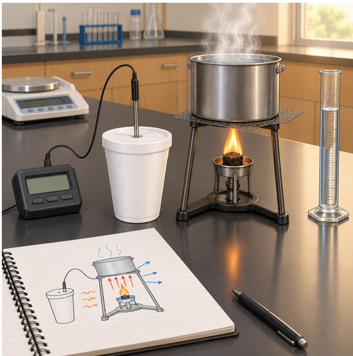
Laboratory bench with a calorimeter, thermometer probe, and combustion apparatus used to measure heat transfer.
