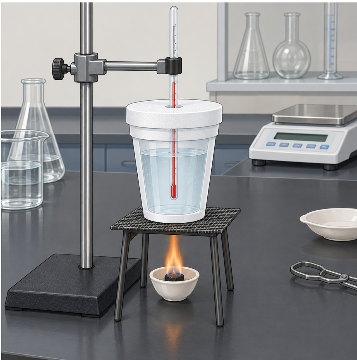
Figure 1: A polystyrene-cup calorimeter setup on a lab bench, showing a thermometer inserted through a cover into a cup of water, a small burning
