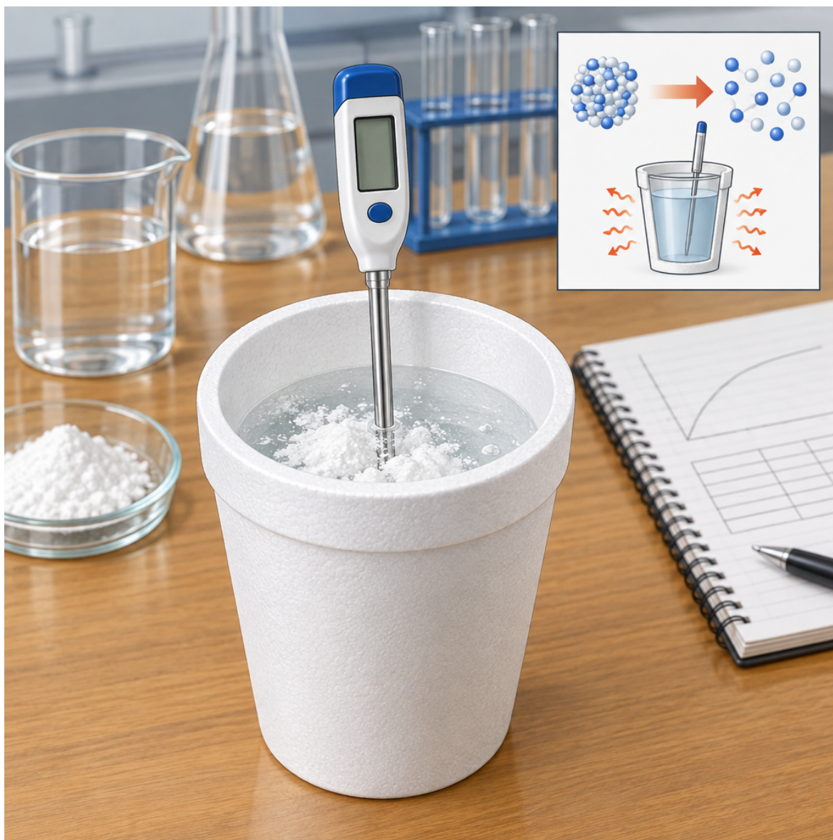
Figure 1: A close-up view of a digital thermometer inserted into an insulated calorimeter cup containing a white powder and clear liquid mixture
