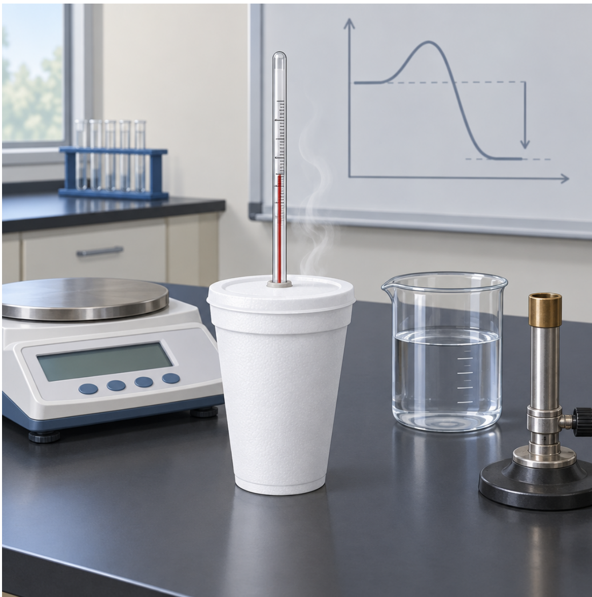
Polystyrene-cup calorimeter with thermometer on a lab bench beside a balance and energy diagram.
