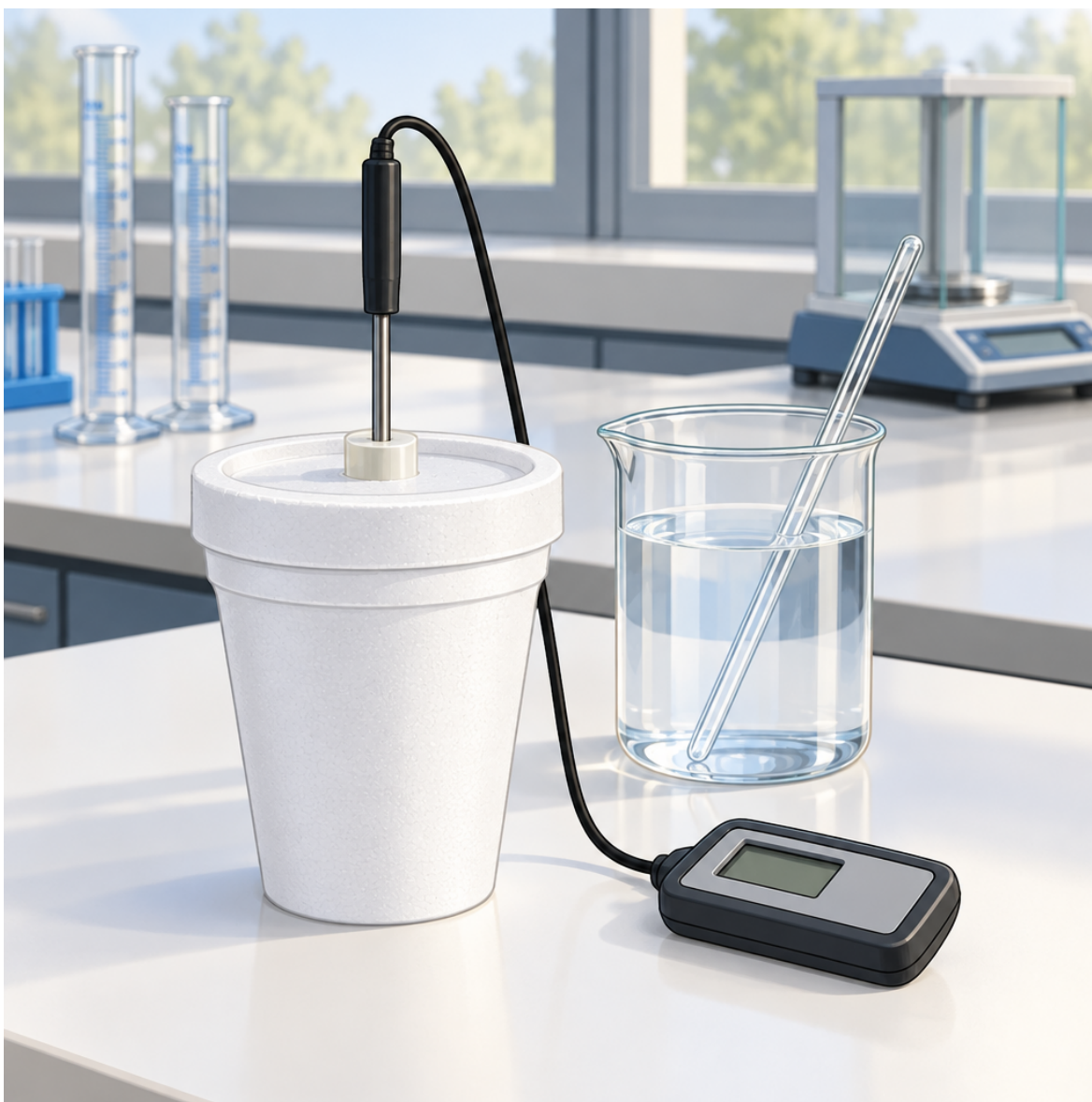
Figure 1: A polystyrene cup calorimeter sits on a white lab bench next to a digital thermometer showing a temperature reading
