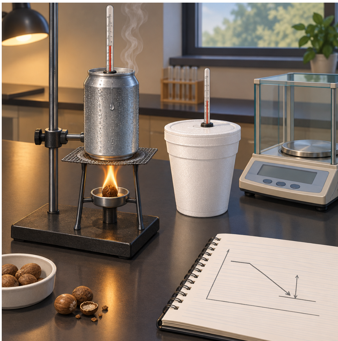
Figure 1: A tabletop laboratory setup shows a small metal stand holding a burning nut sample beneath a soda can filled with water, a thermometer
