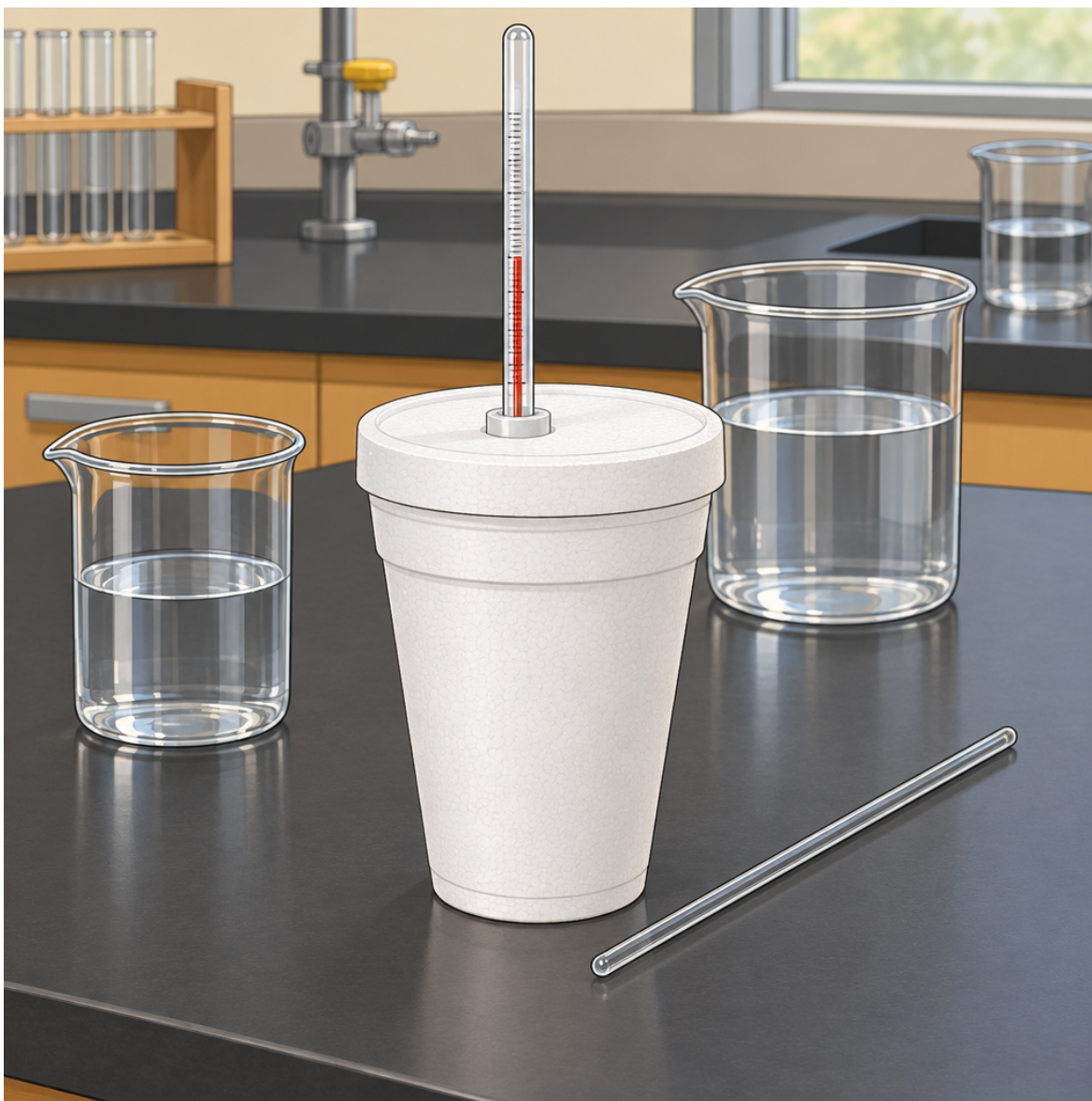
Figure 1: A polystyrene-cup calorimeter set up on a laboratory bench, with a thermometer inserted through the lid and a stirring rod resting beside
