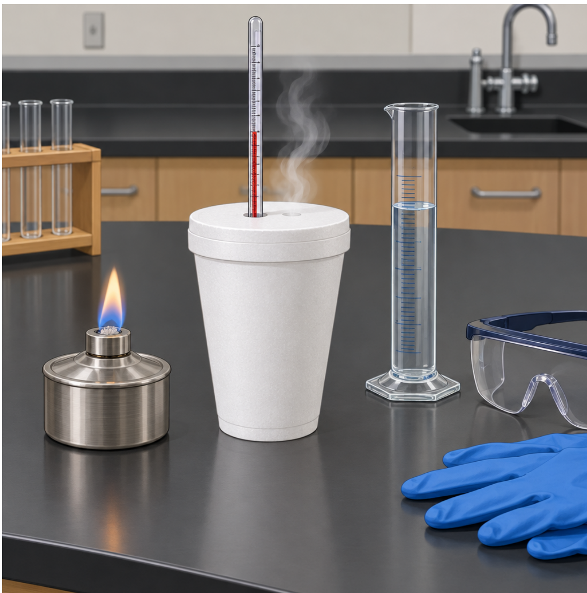
Figure 1: A polystyrene-cup calorimeter sits on a lab bench with a thermometer inserted through the lid, steam rising gently from the opening
