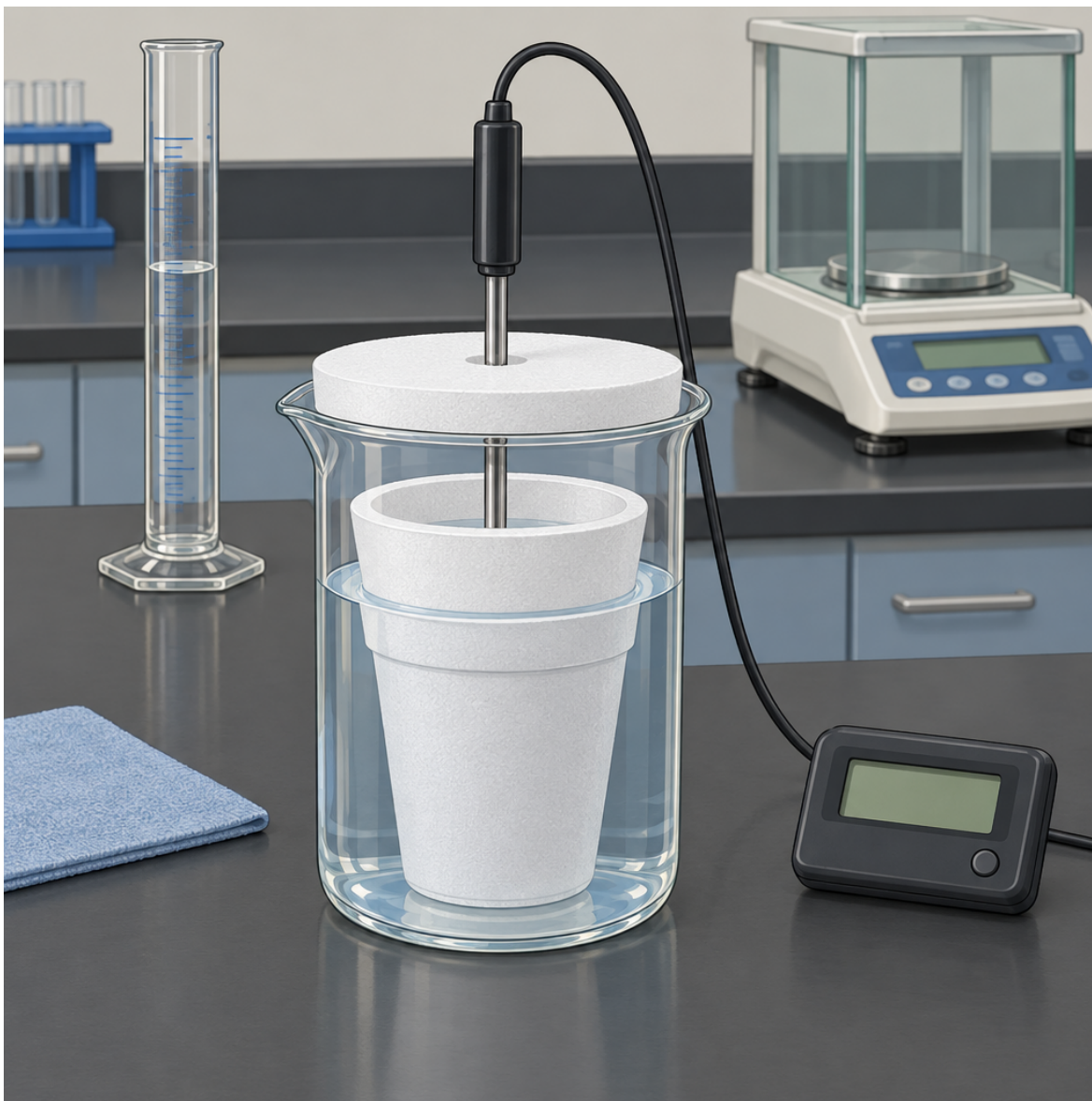
Figure 1: A polystyrene-cup calorimeter setup on a lab bench, showing a nested pair of foam cups inside a beaker for stability, a thermometer probe
