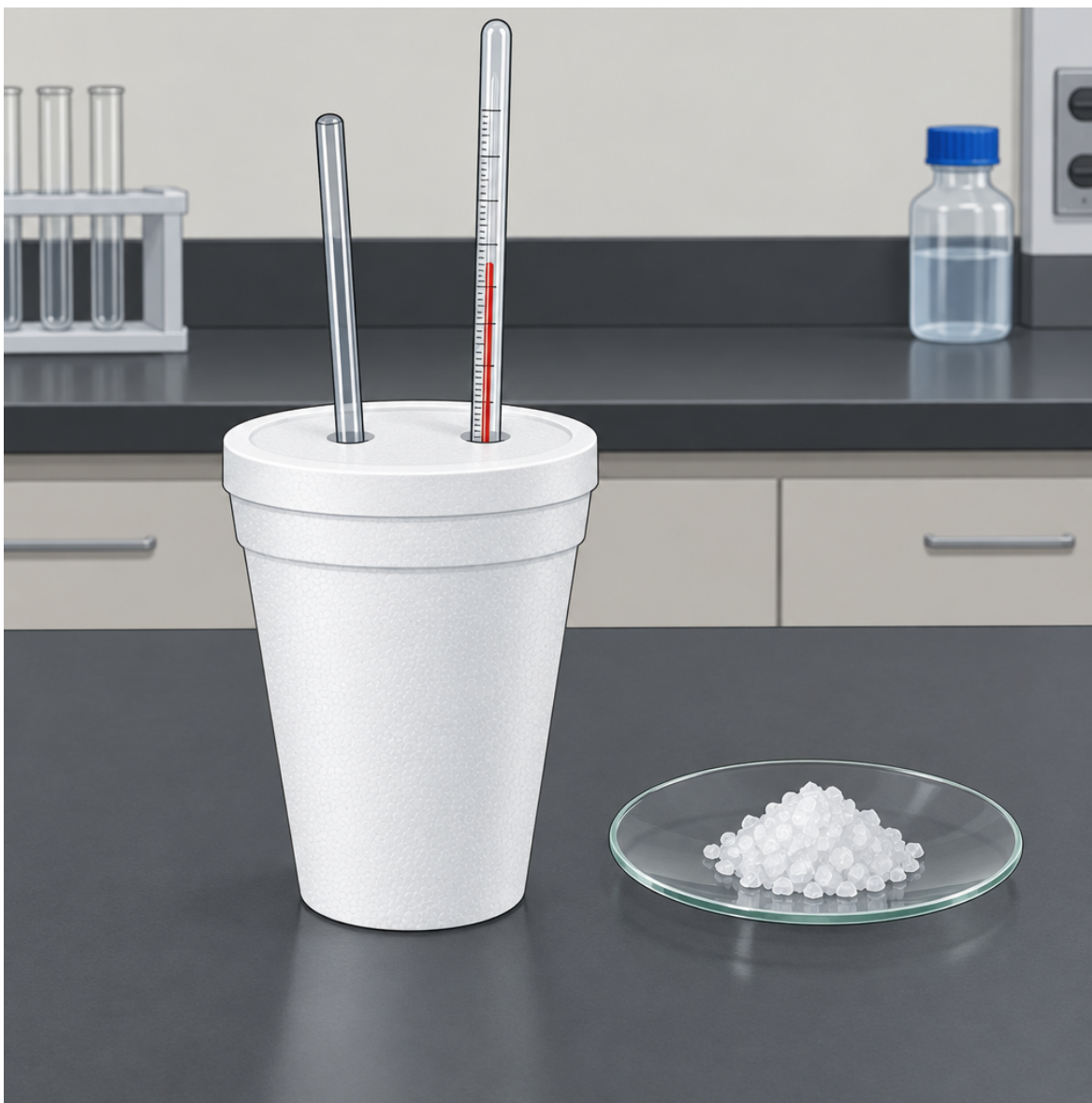
Figure 1: A polystyrene coffee-cup calorimeter sitting on a lab bench, containing a stirring rod and a thermometer inserted through the lid, with a
